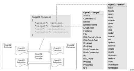
Figure 3 - OpenC2 command structure.
